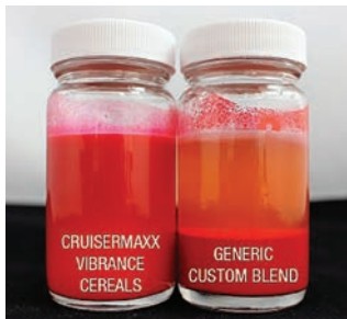
This photo shows slurries of CruiserMaxx Vibrance Cereals and a generic custom blend after 12 hours. There is no product separation with CruiserMaxx Vibrance Cereals. Internal tests at the Syngenta Seedcare Institute; Stanton, Minnesota; April, 2018
